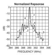
Figure 3. Effect of Interfering Signals on Sensitivity
