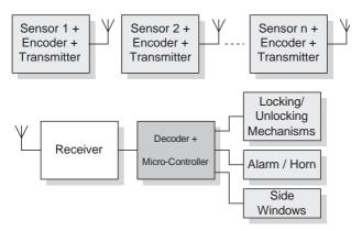
Figure 13. Remote Keyless Entry Application
