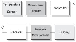
Figure 15. Telemetry Application
